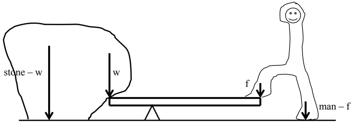
The stone's push towards the ground will be decreased by  $w$  while the man's push with  $f$ . These reduced weights will have their counter forces through the ground, while the  $w + f$  part of the total weights will be equalized through the pivot. So the earth's gravitational counter force will be distributed, but they all come from the weight of the earth by the stone and the man. Finally, a remark:
